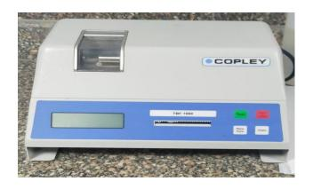
Copley **Friability tester** (dual drum plus abrasion drum), with variable from 20-70rpm  $\pm 1$  rpm with recording timer and it operates at  $10^{\circ}$  angle to test larger tablets
