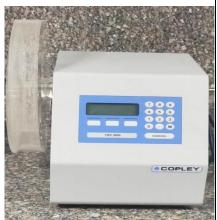
Copley **Tablet disintegration tester** with stroke ,(dual racks)
